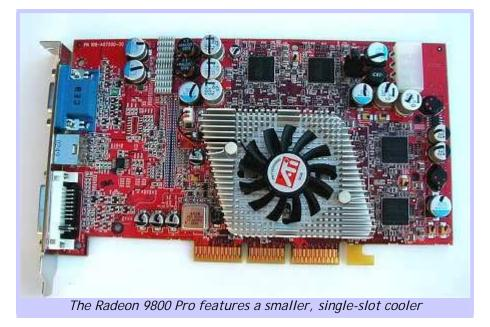
As you can see in the picture above, the Radeon 9800 Pro has a noticably smaller heatsink and fan that fits within a single slot. Subjectively speaking, it is quieter than the GeForce FX and some Radeon 9700 Pro boards. The 128 MB Radeon 9800 Pro lists at US\$399.00 from ATI.
