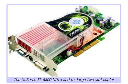
The GeForce FX tested in this review is one of the first commercially available boards, the MSI FX5800 Ultra. It is one of the 100,000 Ultras that will be produced and, as such, features a 500 MHz core clockspeed. For comparison, the normal GeForce FX 5800 runs at 400 MHz, with a memory clockrate of 800 MHz (12.8 GB/s).
