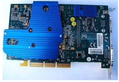
Anyway, this massive heatsink does pay off, as it was significantely cooler than most Radeon 9700 cards after running hours of game benchmarks. Tyan also promises hardware monitoring, but unfortunately our engineering sample did not include this feature.
