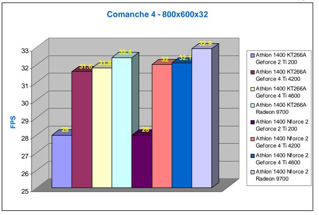
An Athlon 1400 is clearly too slow to show much difference between the Nforce 2 and KT266A. The extra bandwidth of the Nforce 2 goes to waste, as the Athlon 1400 works with a 266 MHz (2.1 GB/s) FSB.
