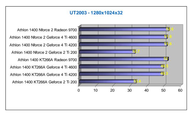
Simply upgrading the motherboard does not help of course, as the Nforce 2 is only slightly faster than the KT266A with a 266 MHz FSB. The step from AGP 4x to AGP8x does not help either. Now let's see the full picture.
