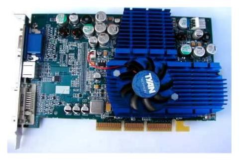
The heatsink consists of two parts, one on the front and one on the back of the card, which give the impression of one massive heatsink.
