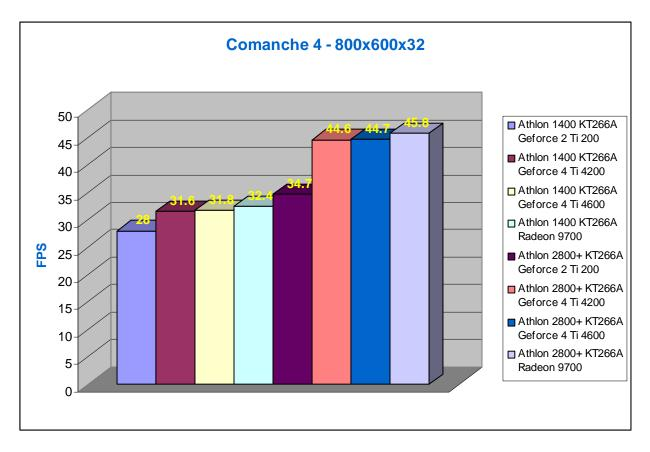
These comanche benchmarks make clear that modern simulators still depend a lot on the CPU, but need some GPU power too. Upgrading the CPU is a decent investment, but only if you have a video card which is based on a GPU a generation more recent than the GeForce 2. Upgrading only the CPU boosts performance by 24%. Not bad, and still a lot better than plugging even the fastest video card in your old rig. When we upgraded the old machine with a Radeon 9700, we saw a meager performance boost of 16%.
