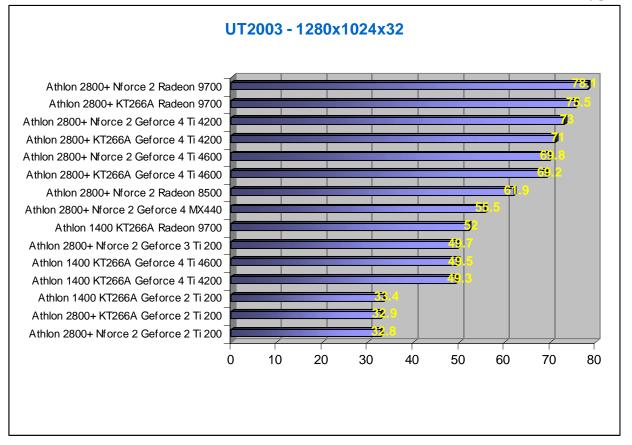
UT2003 likes more CPU power slightly more than video chip power. An Athlon 2800+ with a Geforce 3 Ti 200 comes very close to the Athlon 1400 with a super video card like the Radeon 9700 Pro. Let us pump the resolution to 1600x1200.
