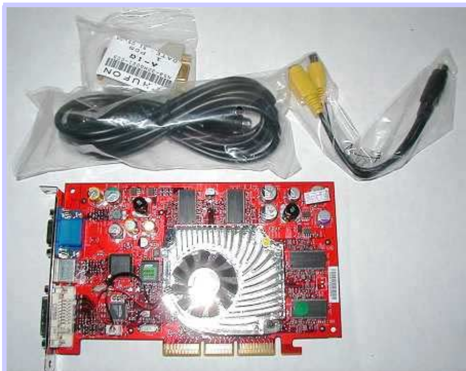
The MSI G4Ti4200-TD64: GeForce 4 Ti4200
