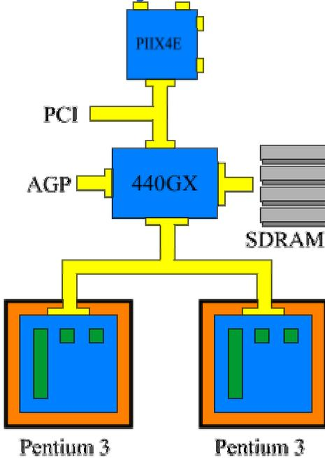
**Chipset architecture:** The main 2-way Pentium III chipset is the 440GX which uses normal SDRAM, though there is also the 840 chipset which uses two Rambus channels (like the 850 Pentium 4 chipset), both of which support up to 4GByte of main memory. The architecture is standard northbridge and southbridge, with the two Pentium IIIs sharing a single bus.
