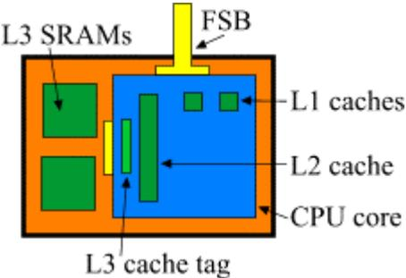
The diagram of a CPU to the left is an example from one of the following pages, and shows a CPU core (the blue box) with some of the features of the CPU core such as the on-die caches. Also shown are some SRAM chips for the external cache that comes in the CPU module (the brown box) for this particular processor, and a connection from the CPU to the rest of the system (the yellow upside-down "T"), often called the FSB - Front Side Bus.
