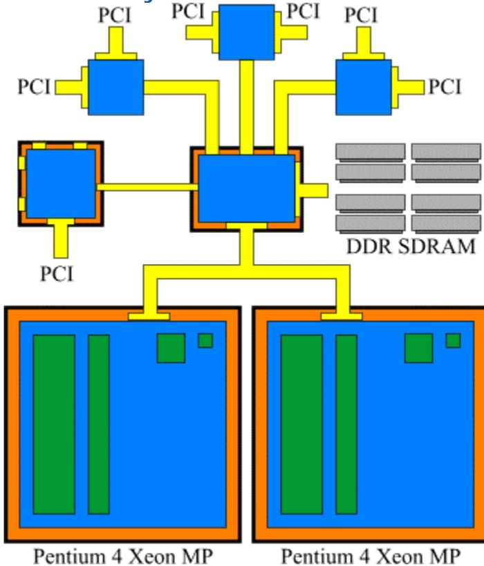
connection to each runs at 566MHz 16-bits wide for 1GByte/s I/O each. It's likely that some of the lower specification dual-processor systems based on this chipset will only use 1 or 2 of the 3 high-speed I/O channels though.
