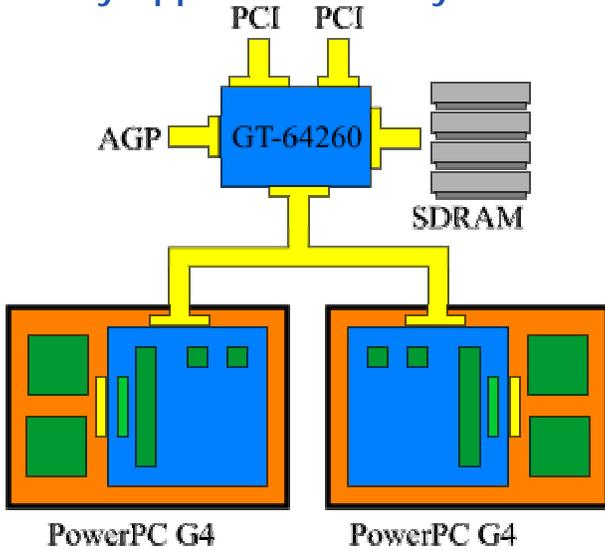
**Chipset architecture:** The basic architecture is similar to Intel's dual processor systems - two CPUs sharing a bus with an ASIC ("GT-64260") that has a memory controller. However, it seems the chipset Apple uses has the southbridge integrated as well, which should save costs, power, size and increase (I/O related) performance a little bit. Up to 1.5GByte/s of SDRAM is supported, though a newer chipset supports up to 2GByte/s of DDR SDRAM.
