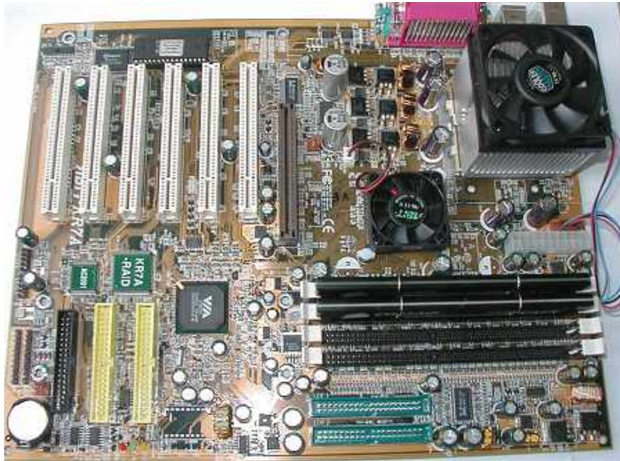
The board supports up to four 1 GB DIMMs for a total memory capacity of 4 GB, but only if you use registered (buffered) DDR modules. Registered modules carry a price premium, though at such module densities, it is not overly significant in our opinion. Crucial currently sells 512 MB PC2100 registered ECC modules for about \$15 more than the equivalent unbuffered, non-parity modules. When using strictly unbuffered modules, the KR7A-RAID is limited to 3 GB.
